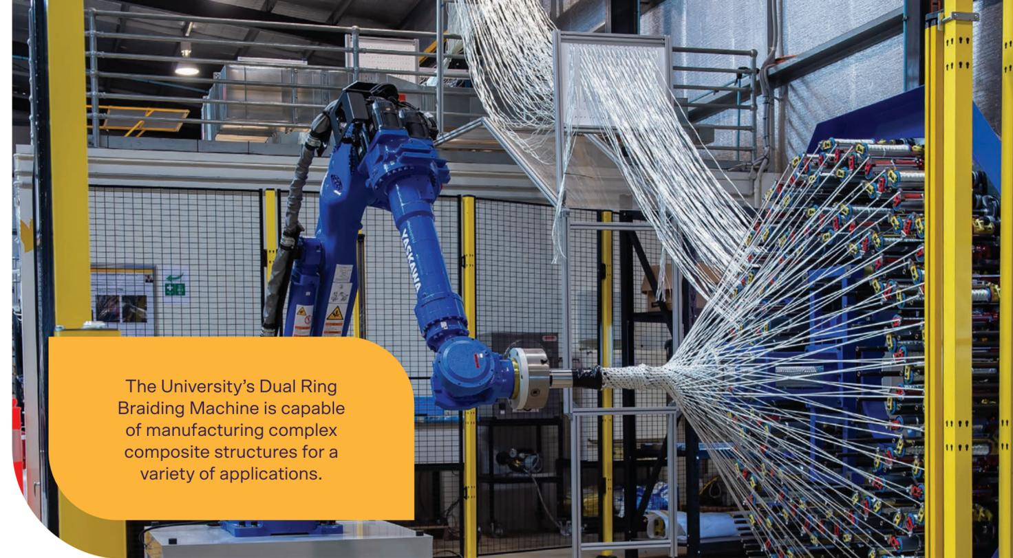
The University's Dual Ring Braiding Machine is capable of manufacturing complex composite structures for a variety of applications.
