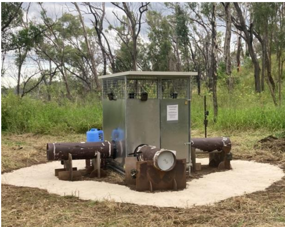
Figure 1. Fully erected vunnel with pipes traps attached (three visible), blue water container, camera traps visible on the star picket in the background and on the front support for the nearest pipe trap (closed). The sand around the completely assembled vunnel and traps is to record tracks of any animals that visit the vunnel.
