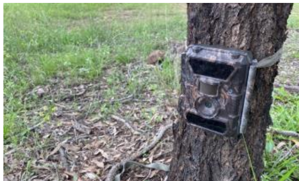
Figure 1: Camera trap placed in situ on a tree and secured with a strap.
